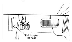
The hood release under the instrument panel
